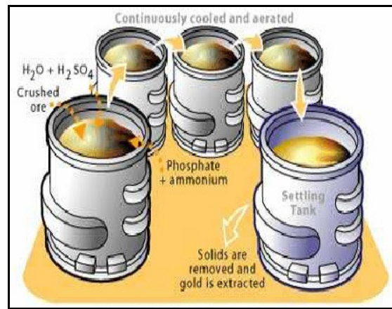
Figure: 3 Stirred tank Biooxidation
