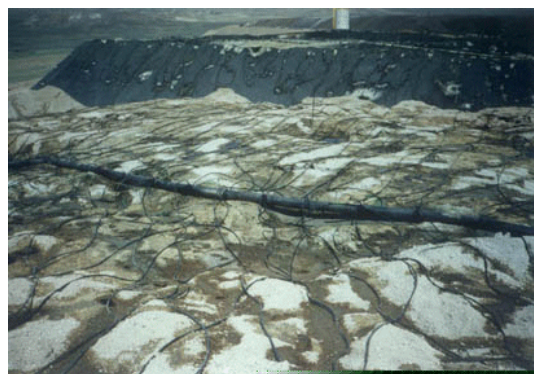
Figure: Top surface of sulfidic-refractory gold bioheap showing drip irrigation with water, sulfuric acid, and biomining microorganisms
