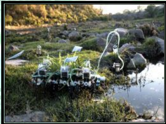
Fig. 14: A robot powered by an integrated microbial fuel cell.
