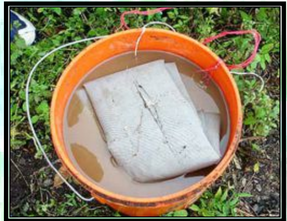
Fig. 15: A cheap microbial fuel cell made by the Lebone group.
