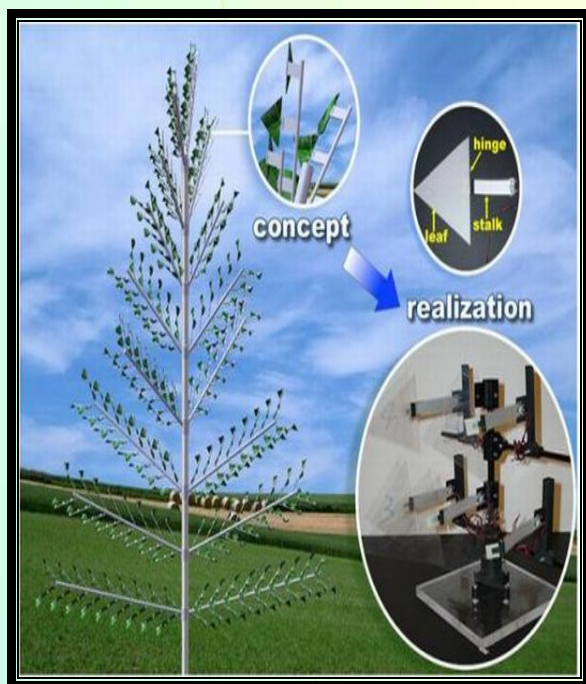
Source: http://heightech.blogspot.in/ Figure: 7 Energy Harvesting 'Piezo-tree' Concept
